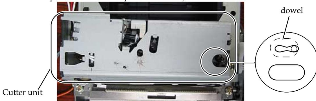
5. When you select partial cut (default), you have to adjust the dowel to the right, as shown. When you select full cut, you have to adjust the dowel to left as shown.
